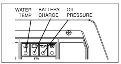
Under normal conditions, when the starter key is turned from [STOP] to [RUN], the BATTERY CHARGING, and OIL PRESSURE monitor lamps will be illuminated. When the engine starts, all the monitor lamps will goes OFF. When fault occurs in running, the corresponding monitor lamp will flash, and the engine will be automatically shut-off.
