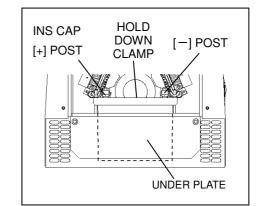
Reinstall a new battery in the reverse order.(Install always the cable to the positive [+] post in the new battery first.)
