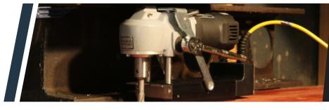
The new HMT RTA40 is a low profile Magnet drill for tight access applications, being designed to fit into any space greater than 200mm. Suitable for use with any standard broaching cutters while optimised to work with the high-performance CarbideMax 40 cutters.
